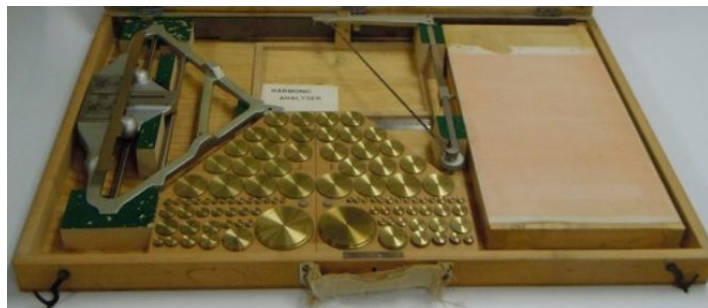
Figure 8: Mader-Ott analyser with two sets of 48 gears [Com2017-1].
