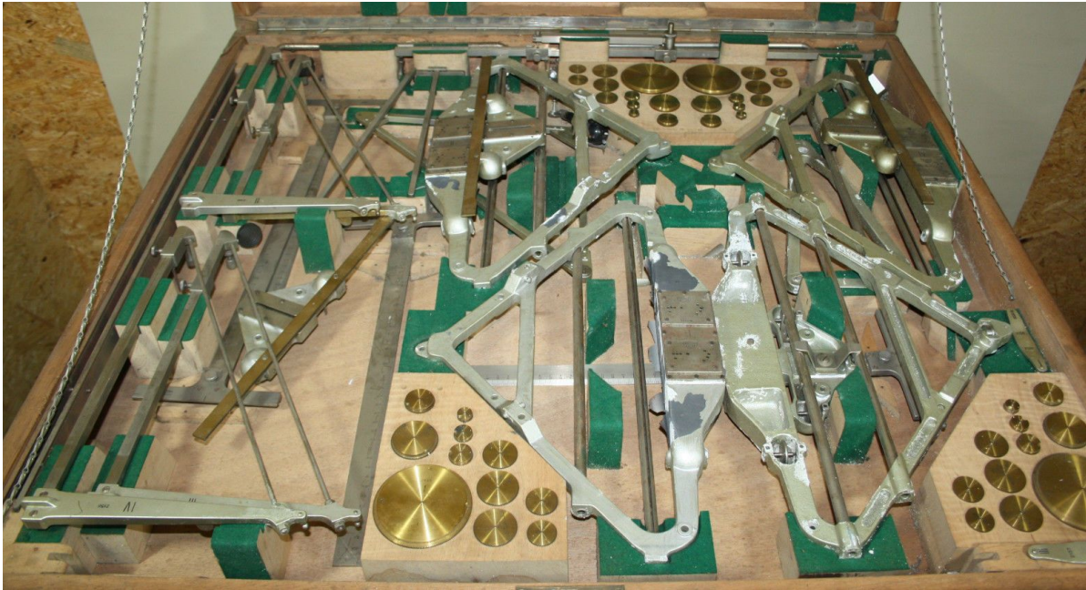
Figure 13: Storage box of Mader-Ott eight-fold harmonic analyser (Serial nos. 2155 to 2158, collection Zerfowski).
