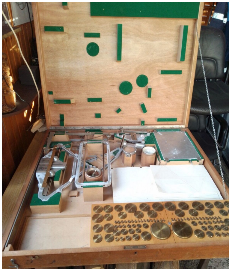
Figure 21: Ott Harmonic Analyser Pewur 218 B Serial Number 2255 including Stieltjes integral extension. Collection Zerfowski.
