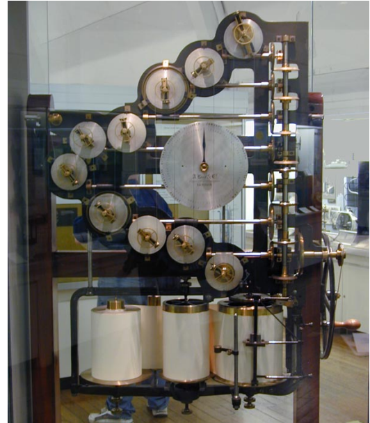
Figure 3: Tidal machine (a harmonic synthesizer) by Thomson (Lord Kelvin) at the Science Museum London. Source: Wikipedia, published by William M. Connolley under Creative Commons License "Attribution-Share Alike 3.0".
