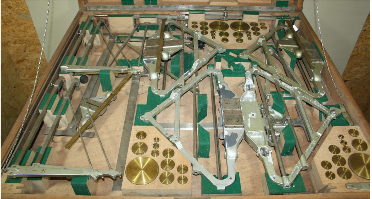
Figure 13: Storage box of Mader-Ott eight-fold harmonic analyser (Serial nos. 2155 to 2158, collection Zerfowski).
