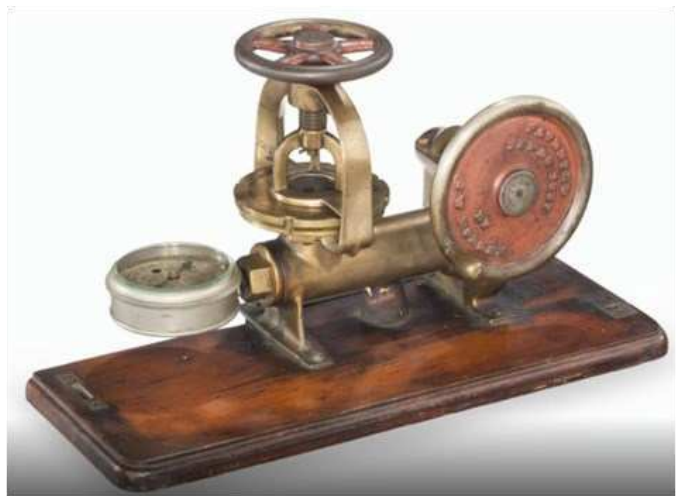
Abbildung 2: Mullen-Tester ca. 1901 (Quelle: https://www.thehenryford.org/collections-and-research/digital-collections/artifact/172160/ )
