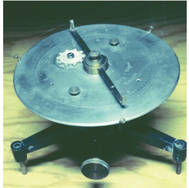
Figure 2. “Sonne's Rechenscheibe” (1878) at the Geodetic Institute, University of Karlsruhe, Germany
